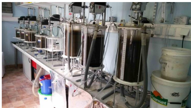
Laboratory tests regarding mono-digestion of corn straw
