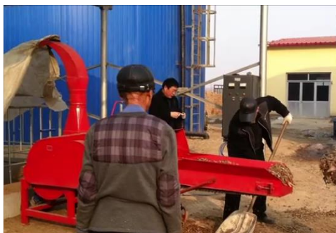
Shredding of the straw
